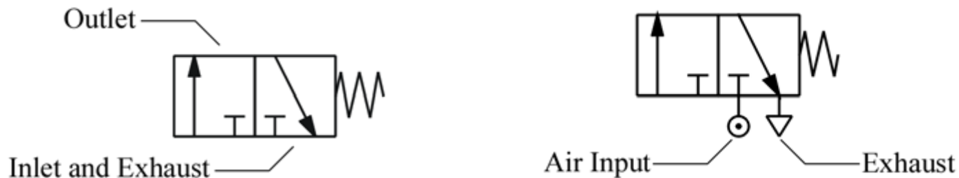
Fig 17 3/2 directional control valve (normally closed type)
