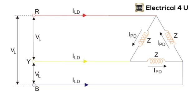
Here,  $I_{LD}$  = Supply Line Current and,  $I_{PD}$  = Winding Current per Phase
