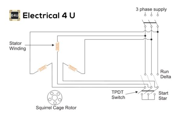
A star delta starter is a type of reduced voltage starter. We use it to reduce the starting <u>current</u> of the motor without using any external device or apparatus. This is a big advantage of a star delta starter, as it typically has around 1/3 of the <u>inrush current</u> compared to a <u>DOL</u> <u>starter</u>.
