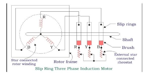
At starting, the resistance is connected to the rotor circuit and is gradually cut out as the rotor pick up its speed. When the motor is running the slip ring are shorted by connecting a metal collar, which connects all slip ring together, and the brushes are also removed. This reduces the wear and tear of the brushes. Due to the presence of slip rings and brushes the rotor construction becomes somewhat complicated therefore it is less used as compare to squirrel cage induction motor.
