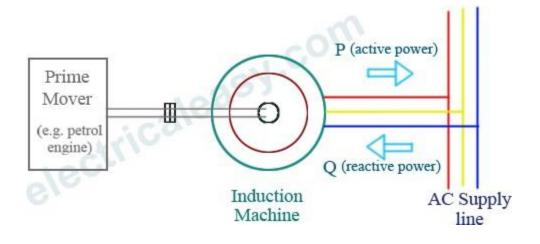
Induction generator is not a self-excited machine. Therefore, when running as a generator, the machine takes reactive power from the AC power line and supplies active power back into the line. Reactive power is needed for producing rotating magnetic field. The active power supplied back in the line is proportional to slip above the synchronous speed. Selfexcited induction generator
