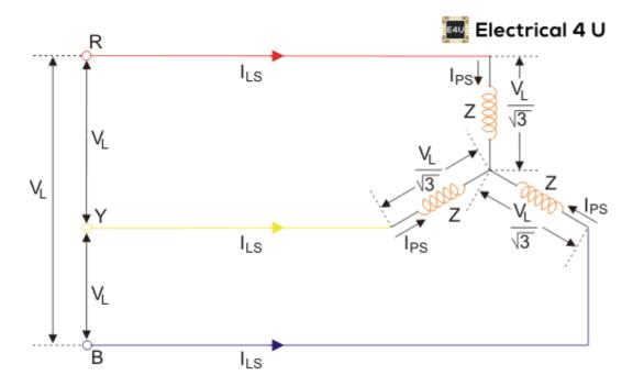
As the winding is star connected, the winding current per phase ( $I_{PS}$ ) equals to supply line current ( $I_{LS}$ ).
