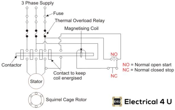
If we press the stop button, the current through the contact becomes discontinued, hence supply to the motor will not be available, and the similar thing will happen when the overload relay operates. Since the supply of motor breaks, the machine will come to rest. The contactor coil (Magnetizing Coil) gets supply even though we release start button because when we release start button, it will get supply from the primary contacts as illustrated in the diagram of the **Direct Online Starter**.
