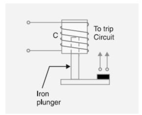
> When a fault occurs the current through the relay coil becomes more than the pickup value, causing the plunger to be attracted to the solenoid. The upward movement of the plunger closes the trip circuit, thus opening the circuit breaker and disconnecting the faulty circuit.
