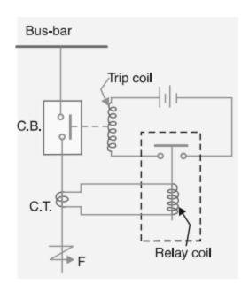
The relay circuit connections can be divided into three parts
