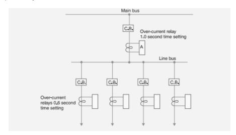
➤ If the faults are not cleared by primary relay system because of trouble within the relay, wiring system or breaker. Under such conditions, back-up protection does the required job.
