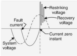
At current zero, a high-frequency transient voltage appears across the contacts and is caused by the rapid distribution of energy between the magnetic and electric fields associated with the plant and transmission lines of the system. This transient voltage is known as restriking voltage.
