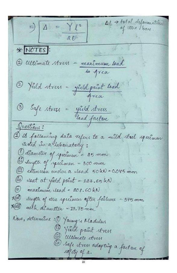
$\Rightarrow$  given: d = 25 mm l = 300 mmP = 50 kN = 50×103 N Al = 0.045 mm yield point load = 127.65 kN = 127.65 × 103 N maximum laad = 208.60 kN = 208.60 × 103 N uload factore = 2. ( De Pe  $=) E = \frac{P\ell}{AA\ell}$   $=) E = \frac{P\ell}{AA\ell}$ and doing and the
