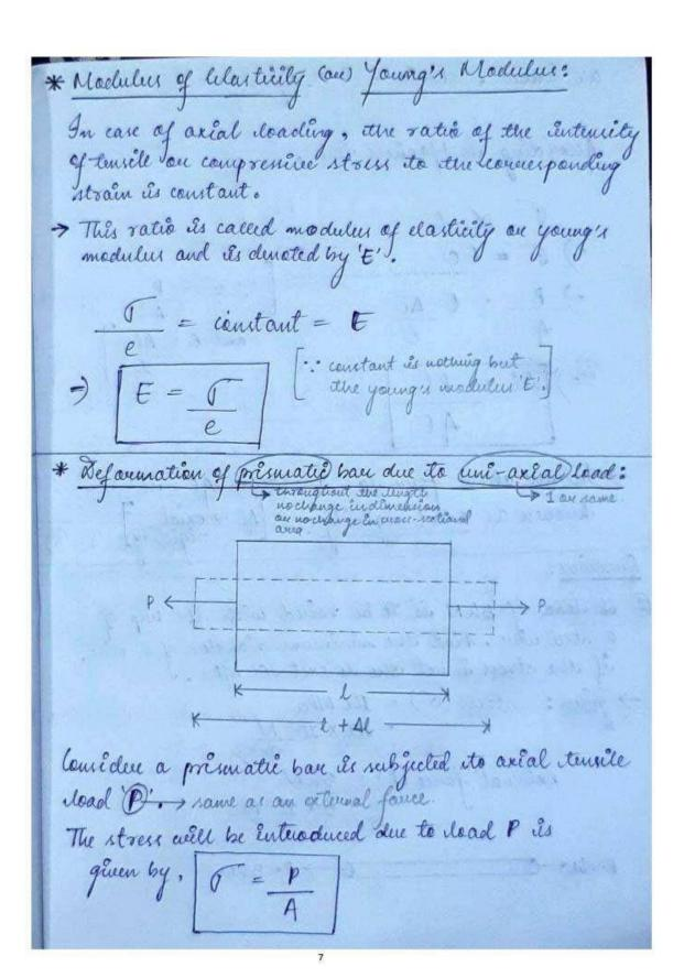
une huou , strain : l = <u>Al</u> According to Hooke's clave, ME) TAL = PL -> In the above foundla, the teum At' is hueven as axial rigidity. At - axial rigidity Questions: @ A load of 5kN is to be raised with the help of a steel usur. Find itte minimum dianeter of a wine, if the stress is not the to exit 100 MPa. I  $\rightarrow g_{\underline{uen}}$ : stress (6) = 100 MPa = 100 x 10  $\frac{6}{m^2}$ . external force (1) = 5kN = 5 x 103 N P=5WX O
