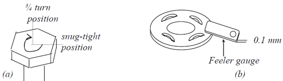
Figure 10.7 Tightening of HSFGB bolts
